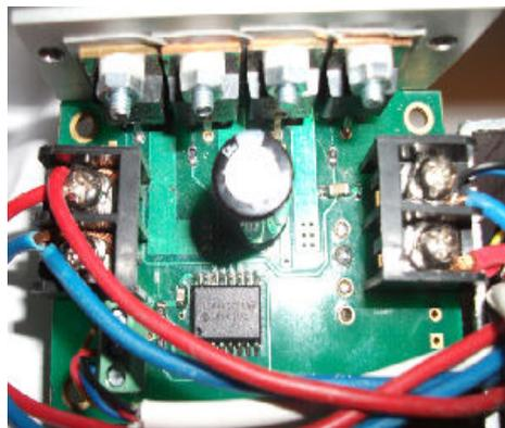
Fig.10. H-Bridge used in the system
