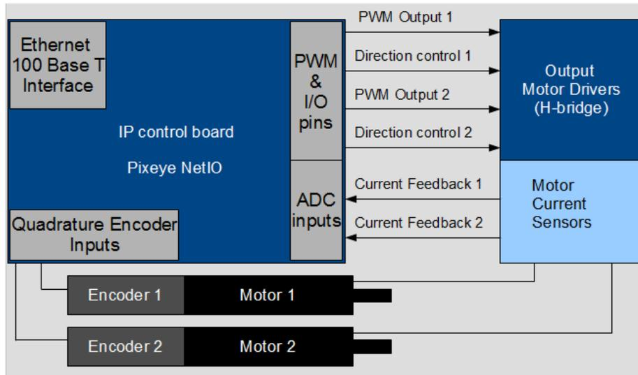
Fig.11: Control system for differential drive mobile platform
