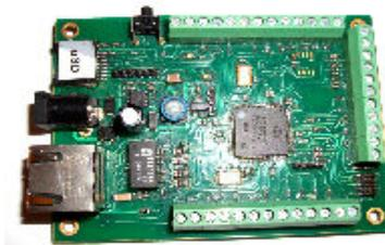
Fig.5: The Net IO control board
