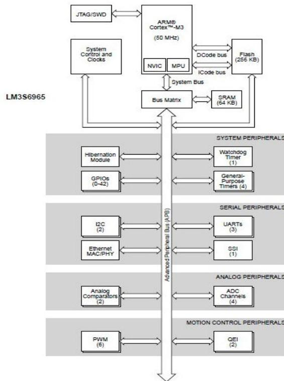
Fig.6: Internal structure of LM3S6965
