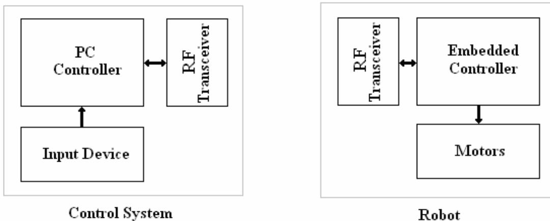
Fig. 3 Soccer Robot Control System
