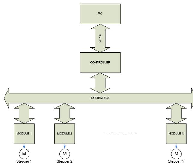
Fig. 2 Control System of Educational Robots – ROBCO SCARA
