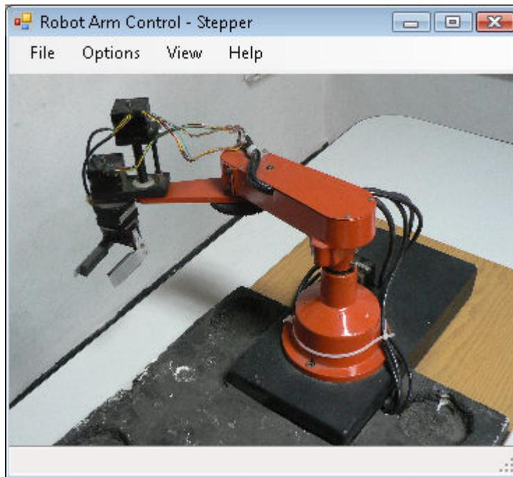
Fig. 3 ROBCO SCARA Graphical User interface
